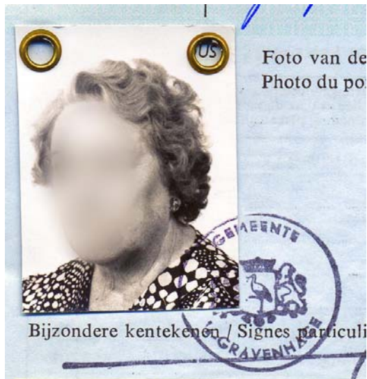
Figure 8 – Example of the application of tubular rivets and an ink stamp to bind a photo to a Dutch passport identity page.
