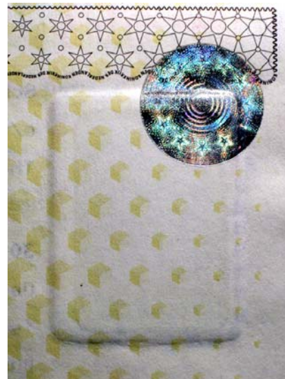
Figure 9 – The successor of the “black rag”, was issued in 1995 and lasted until 2001. It still had a separate passport photo, which was protected by a 3M Confirm cover foil. On the back of the holder page (shown here) a kinegram was applied over a corner of the photo, as a further protection against photo swapping. To no avail, because it did not at all stop successful photo swapping. The passport had a red cover and was soon called “the red dud”.
