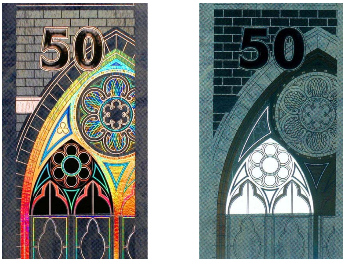
Figure 13 – STRAP Perfection with zero.zero® technology (19 x 33 mm detail): in first order diffraction (left) and in transmission (right), showing register between demetallized diffractive foil and transparent OVD windows. Foil width 16 mm. (Sample courtesy of Leonhard Kurz GmbH & Co. KG, Germany).
