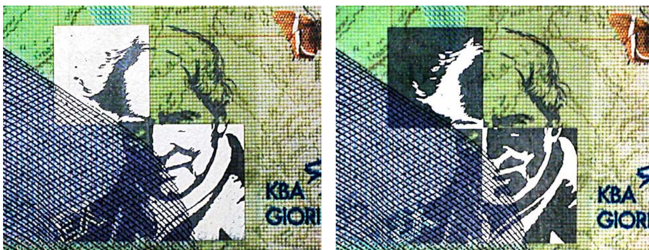
Figure 14 –Kurz Modular Banknote Concept with zero.zero® technology (detail 20 x 24 mm): register between printing and a diffractive foil with achromatic blazed gratings ( white diffractive watermark ) illuminated from top (left) and illuminated from bottom (right). (Sample courtesy of Leonhard Kurz GmbH & Co. KG, Germany).
