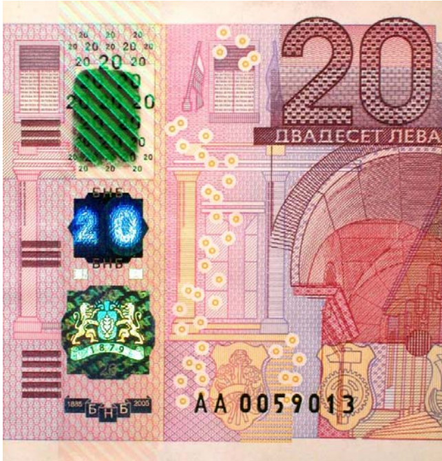
Figure 15 – Verifeye® transparent window feature in the 20 Leva Bulgarian paper-based commemorative note (2005): in diffuse reflection including first order diffraction (left) and transparent window details (15 x 25 mm) in transmission in RH circularly polarized light (center) and LH circularly polarized light (right).
